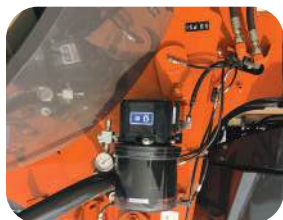
Automatic Lubrication System (ALS)
