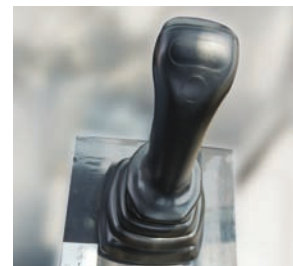
Smooth bucket and arm control with pilot lever
