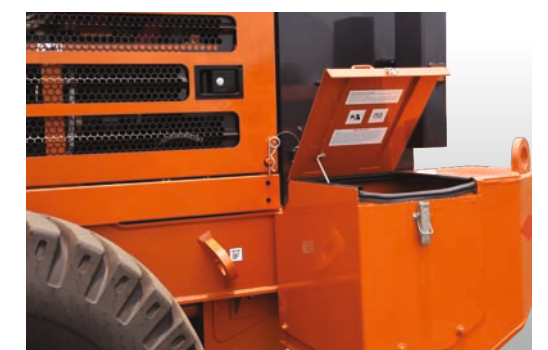
Side covers for easy access to batteries
