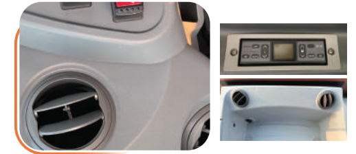
Heating, Ventilation, and Air Conditioning (HVAC)
