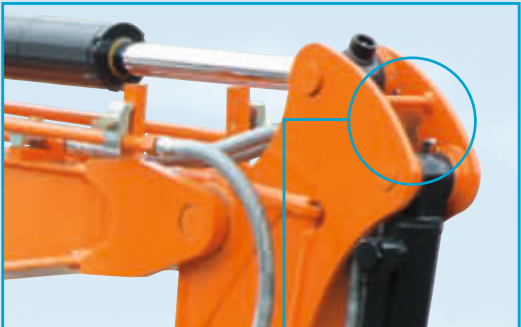
Hydraulic hose guard Bucket cylinder hoses are placed inside the arm thereby protecting the hoses
