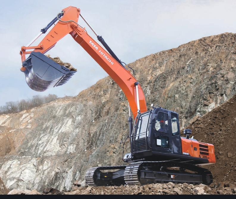
Engine Power: 131 HP @ 2000 rpm | Operating Weight: 20,100 - 20,300 kg | Bucket Capacity: 0.9 - 1.7 m<sup>3</sup>
