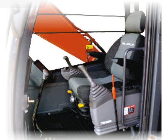
Ergonomically designed spacious cabin with comfortable suspension seat and air lumbar support
