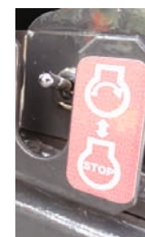
Emergency engine stop switch
