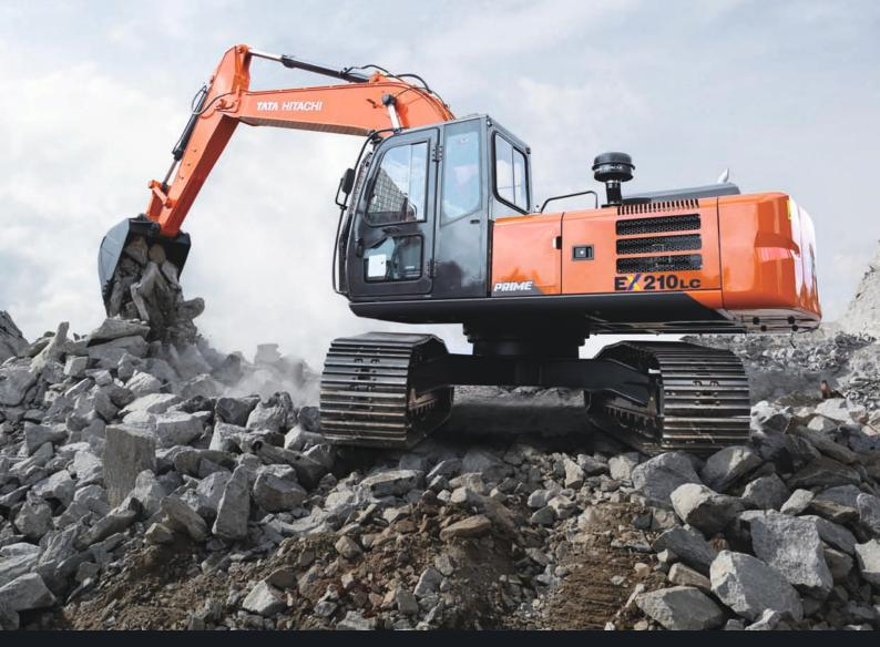
Model code: EX210LC-5G | Engine Power: 131 HP @ 2000 rpm | Operating Weight: 20,600 - 20,800 kg | Bucket Capacity: 0.9 - 1.7 m<sup>3</sup>
