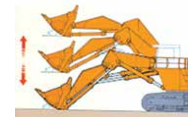
Auto Bucket level raise system
