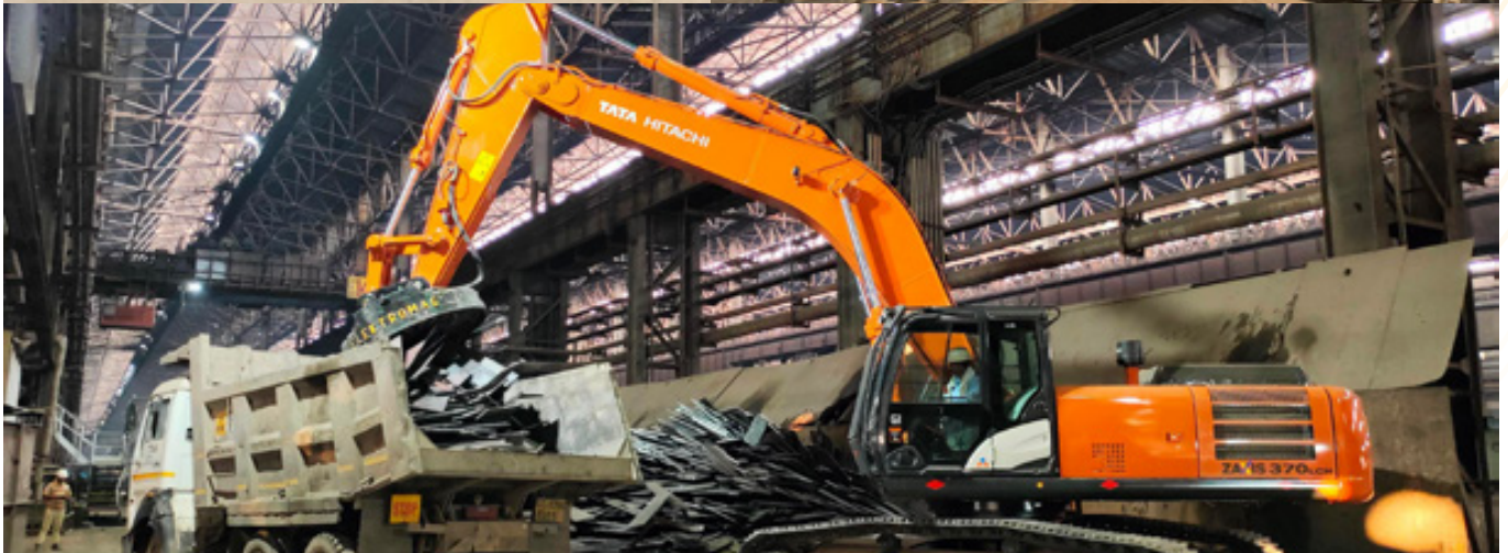
Installed 1st magnet 30 Ton model, LMR 160 L in machine model ZX 370 LCH GI at Ms Ferro Scrap Nigam Ltd, Bhilai steel plant campus
