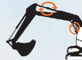
Boom & Arm Regeneration resulting in energy saving
