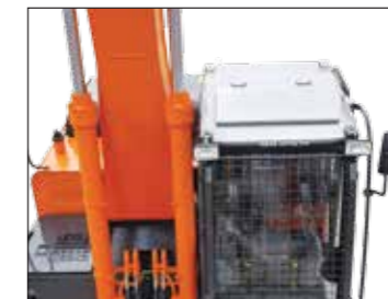
Heat reflective coating on cabin top
