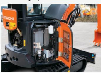
Air pre-cleaner ensures longer life of filters and reduces maintenance cost
