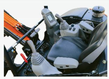
Lowering Lock lever is compulsory for engine start function
