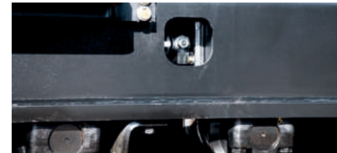
Adjuster greasing hole repositioned to reduce dirt accumulation
