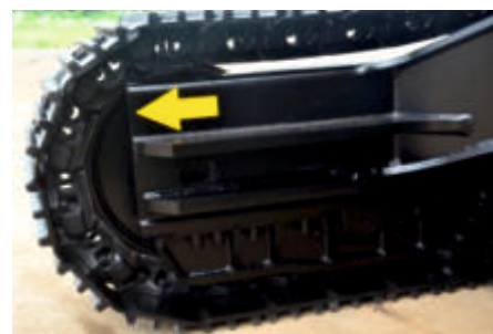
Reinforcement at idler side
