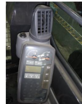
The panel is aptly positioned within the natural line of sight so as to ensure that all key operating conditions can be monitored with just a glance.
