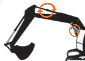
Boom & Arm Regeneration resulting in energy saving
