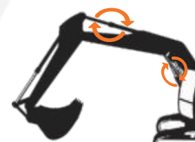
Boom & Arm Regeneration resulting in energy saving
