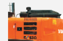
Honeycomb mesh type ROC door
