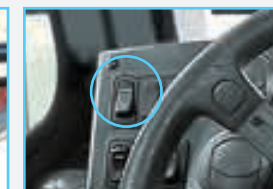
Screen Changeover Switch
