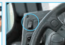
Screen Changeover Switch
