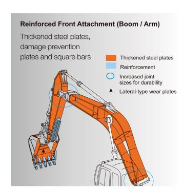
The boom top and bottom are strengthened using high tensile steel and through increase in dimensions of bosses. The boom and arm joints incorporate steel bushings to enhance durability. Steel plates of higher size and thickness are used in the arm to make it stronger and more rigid. Special flange type arm bucket bushes ensure that there is no direct rubbing of arm and bucket bosses, thereby increasing the life of pins and bushes substantially.
