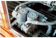
Hydraulic oil is filtered at high pressure to remove damage-causing contaminants. This filter is positioned down-line from the pumps to help prevent damage in the rare event of pump failure. Positioned for easy maintenance.
