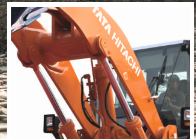
Increased lift arm torsion improves productivity.
