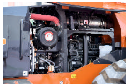
Easy access for ground level maintenance.
