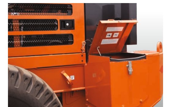
Side covers for easy access to batteries
