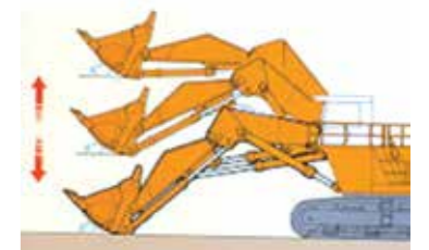
Auto Bucket level raise system
