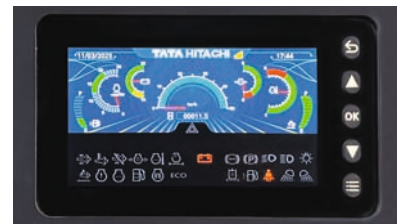
Multi-color monitor for fuel, urea, speed, and more
