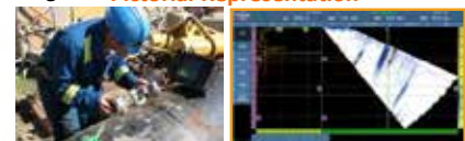
A person performing PAUT inspection and output image
