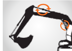
Boom & Arm Regeneration resulting in energy saving
