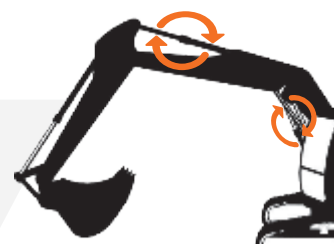
Boom & Arm Regeneration resulting in energy saving
