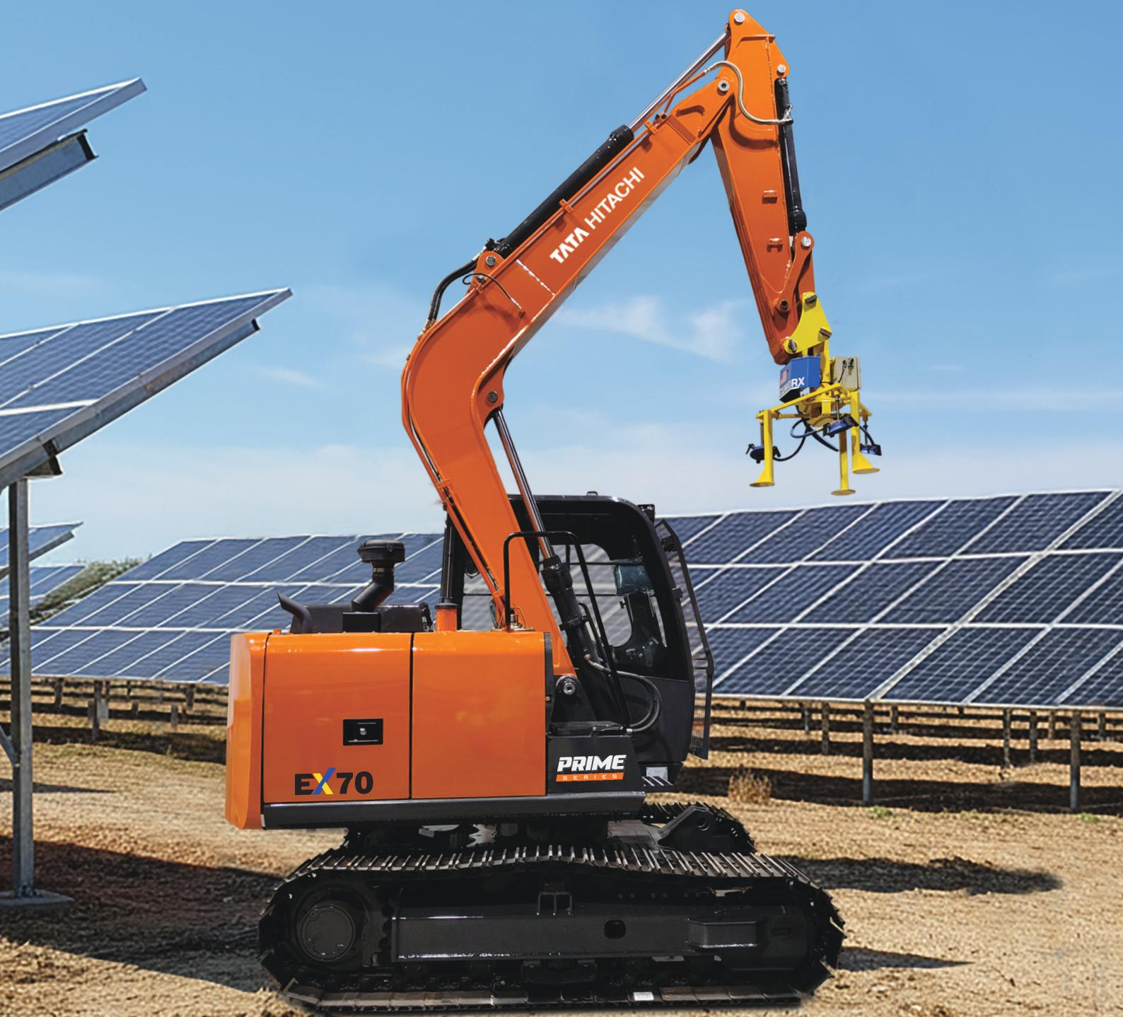
The Solar Panel Lifter system allows easy installation and manipulation of solar panel modules in the field via attachment to a variety of mini-excavators. This system reduces worker fatigue and wind gust concerns, increases worker safety, and gently handles the delicate modules.
