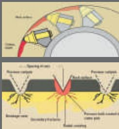
More than the performance of the cutter (kW), it is the pick force and cutting head torque which creates the optimal cutting operation.
