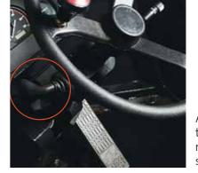
A lever used to set machine travel direction (forward or reverse). Machine will only start if it is in neutral position.
