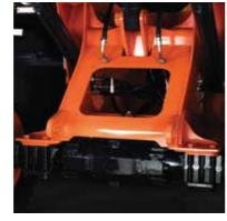
The new design with access cutout in the front frame provides easy access to hydraulics. Also hydraulic pressure measurement ports are conveniently located for hydraulic troubleshooting.
