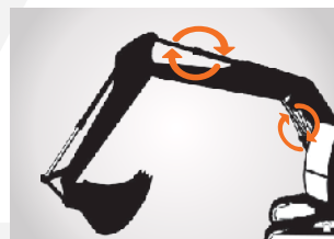
Boom & Arm Regeneration resulting in energy saving
